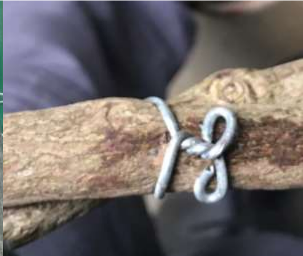
Fig. 138. Safe wire ends
